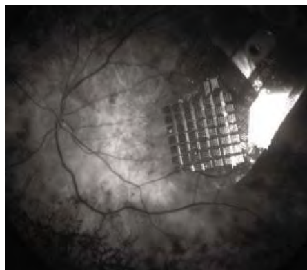
Chip in the eye. IMI's implant sends visual data via gold wires to a tiny electrode array tacked onto the human retina.
